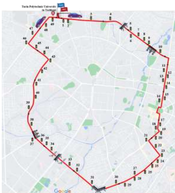
Figure. 4. Testing start-stop system in the Tashkent city.
