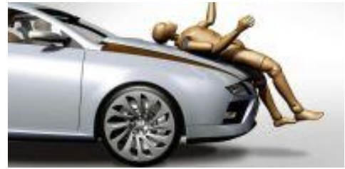
Fig. 6. Opening the hood in a collision with a pedestrian
