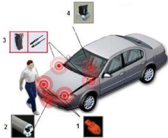
Fig. 4. The scheme of the pedestrian protection system: 1 - acceleration sensor; 2 - contact sensor; 3 - hood lift; 4 - control unit
