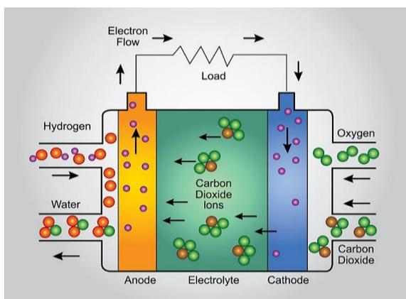
Fig. 1. Molten carbonate fuel cell. [5]
